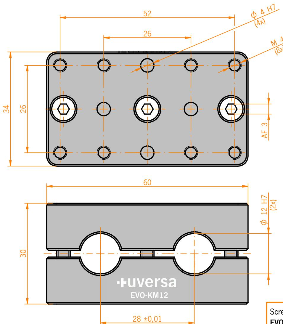
Screw-on borehole diagram valid for:
